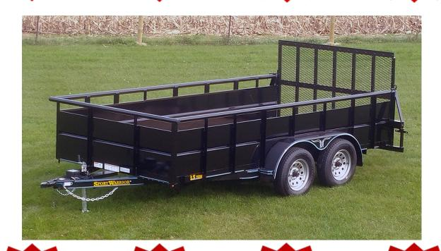
2 X 8 Treated Pine Floor 30" High Metal Sides Pipe Top Rail Set Back Rapid Jack
