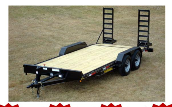
Heavy Duty Treadplate Steel Fenders Solid Bump Bar w/ 14 Stake Pockets 7,000# Dropleg Jack Structural Channel Main Frame
