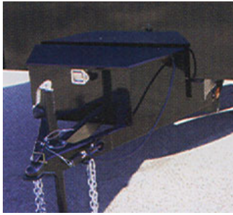
Hydraulic System in Lockable Box
