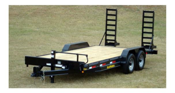
Heavy Duty Treadplate Steel Fenders Solid Bump Bar w/ 14 Stake Pockets
