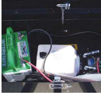
12V hydraulic pump in lockable tongue box
